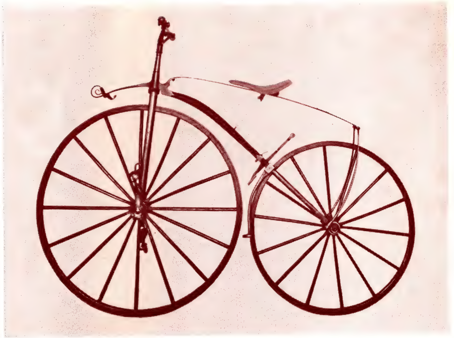
FRENCH VELOCIPEDE , produced by Pierre and Ernest Michaux in Paris in 1863, was the first commercially important machine on the way to the modern bicycle. The "bone-shaker," as the vehicle was sometimes called, had cranks with pedals fixed directly to the hub of the front wheel and hence suffered from the limitation of having too low a gear ratio.
