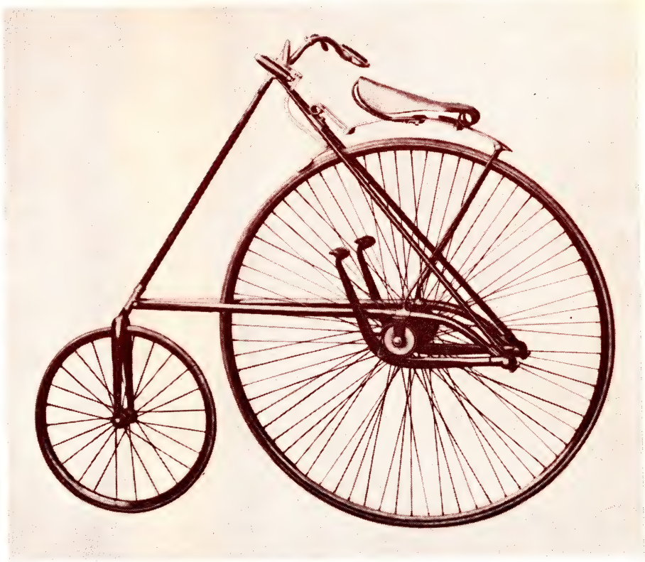
STAR BICYCLE, built by the Smith Machine Company of Smithville, N.J., in 1881, was another notable attempt to make the high-wheeler safer. The machine had a small wheel in front and used a system of levers, drums and straps to drive the large wheel at the rear.
