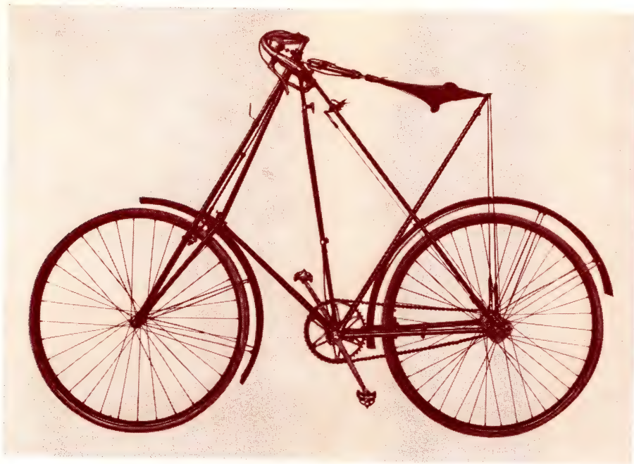
FULLY TRIANGULATED FRAME was the most distinctive feature of the Dursley-Pedersen bicycle, which achieved some success in England in the 1890's. This machine used small-diameter tubes in pairs and was remarkably light, weighing in at only 23 pounds.
