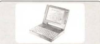
CPU 80386SL/25, 2 MB RAM (ESPANDIBILE A 8 MB), FDD 1.44 MB, HDD 60 MB, DISPLAY 10" 64 TONI GR., PORTA SERIALE E PARALLELA, PESO KG. 2.5, BATTERIA, MS-DOS 6.0, WINDOWS 3.1 LOTUS ORGANIZER.
